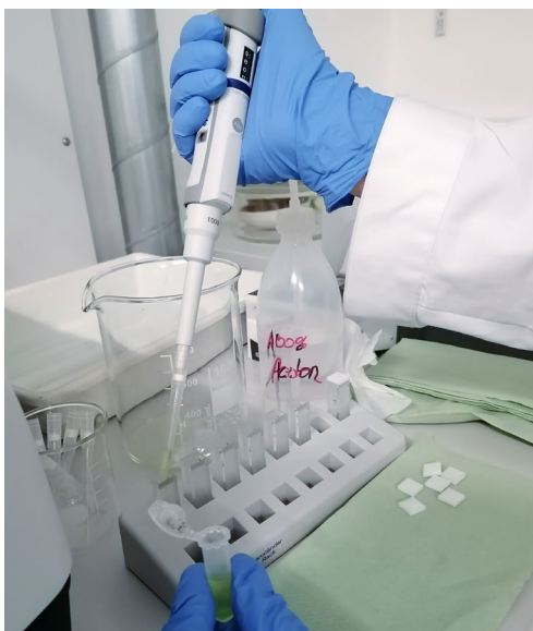
One methodology that complemented the molecular methods was the extraction of chlorophyll a and b. Chlorophyll was extracted by acetone and the extract was transferred from reaction tubes to cuvettes to be measured with a spectrophotometer. (Photos: Tränkner)
