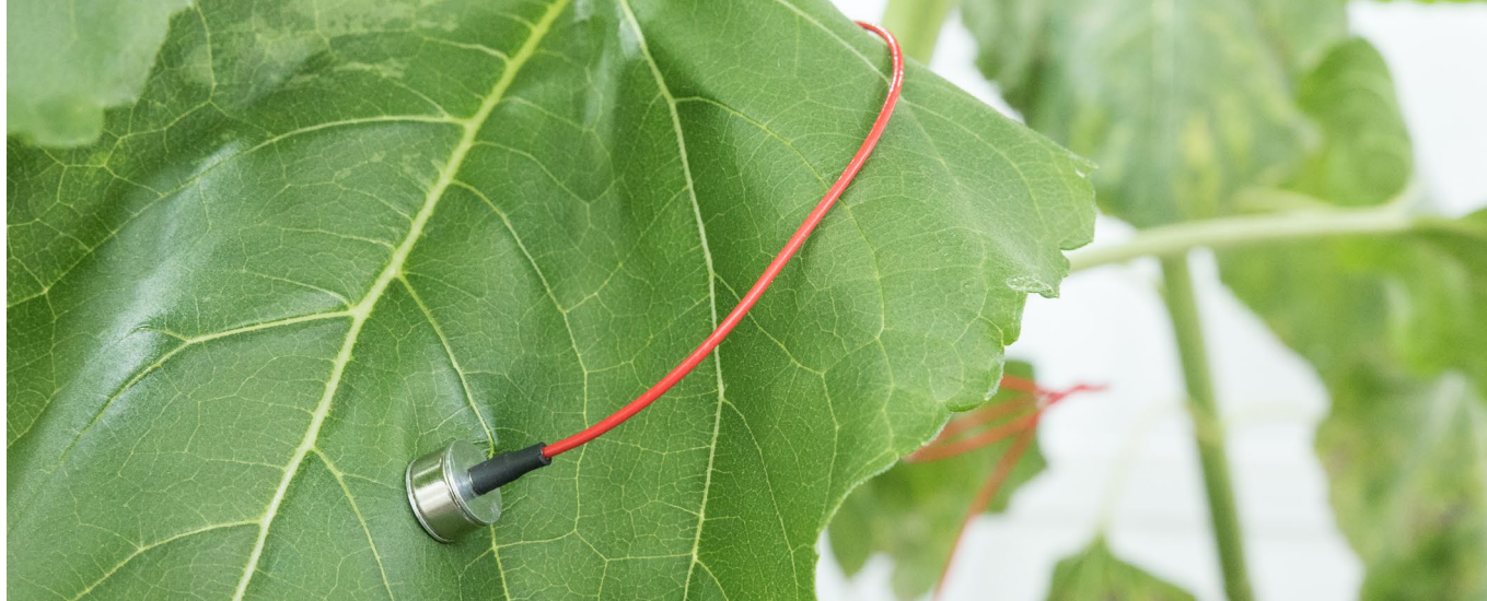
Assessing leaf turgor pressure and water status in sunflower at IAPN using a LPCP probe. (Photo: D. Jákli)
