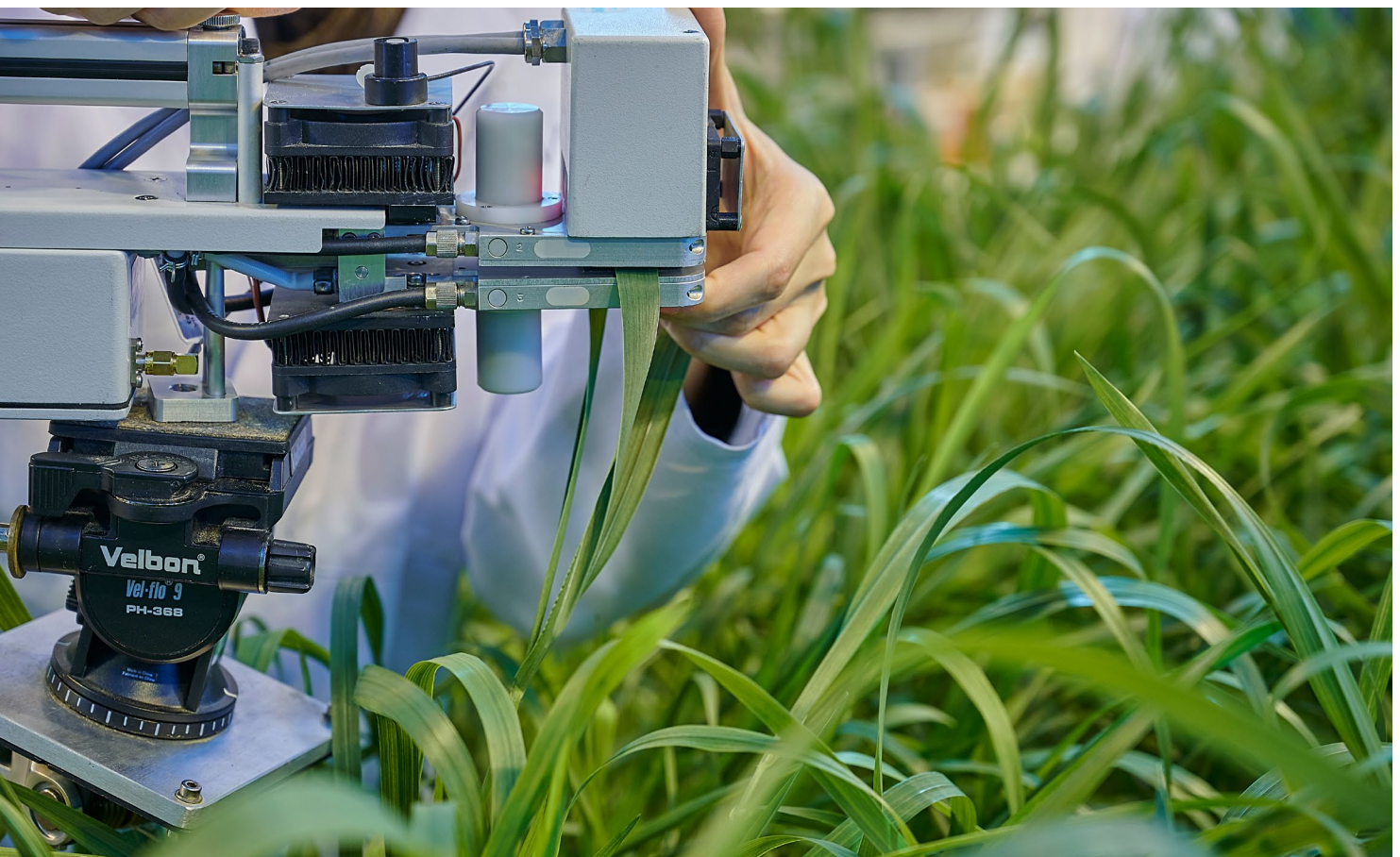
Assessing the photosynthesis of wheat by the measurement of leaf gas exchange in an IAPN experiment. (Photo: K+S)
