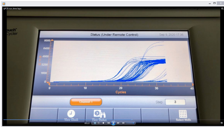
The run of a quantitative real-time PCR (qPCR) was recorded and a time lapse video was created, so that the students were able to see the full analysis of their samples. (Source: Jamali Jaghdani)
